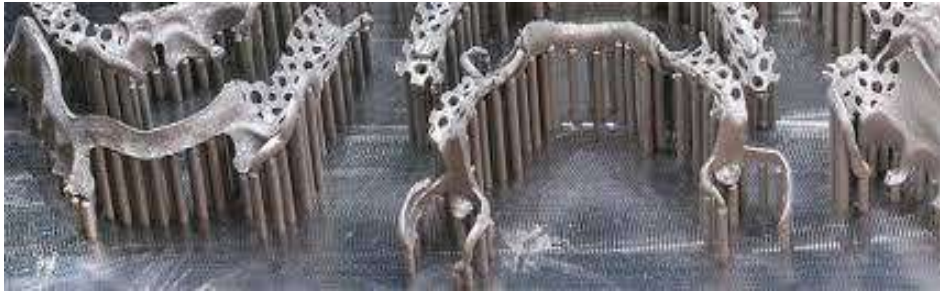
Metal frame 3D printed
